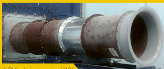
A TA fan being tested in AMCA
