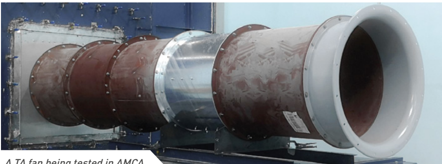
A TA fan being tested in AMCA
