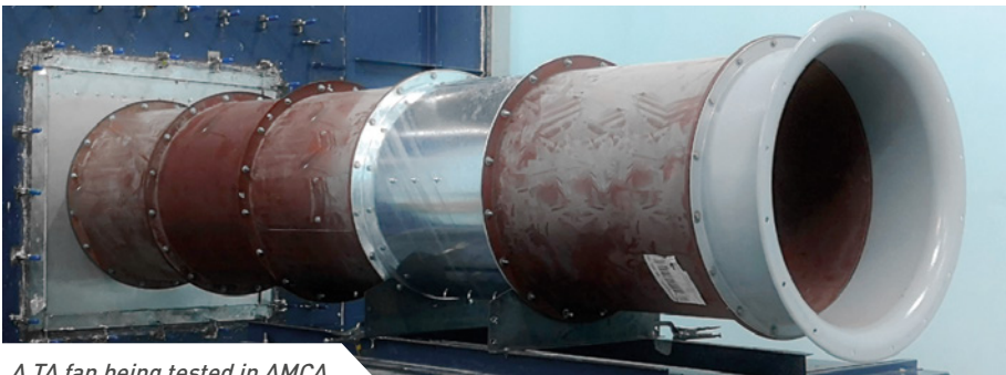
A TA fan being tested in AMCA
