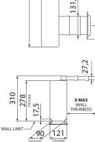
In case of wall thickness < to the measures indicated it is sufficient to cut the extensions or spigots on site.
