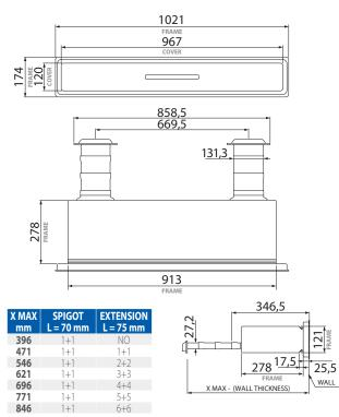
In case of wall thickness < to the measures indicated it is sufficient to cut the extensions or spigots on site.
