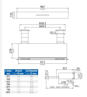
In case of wall thickness < to the measures indicated it is sufficient to cut the extensions or spigots on site.
